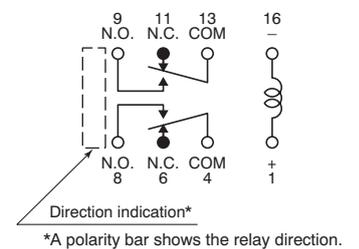
\*A polarity bar shows the relay direction.
