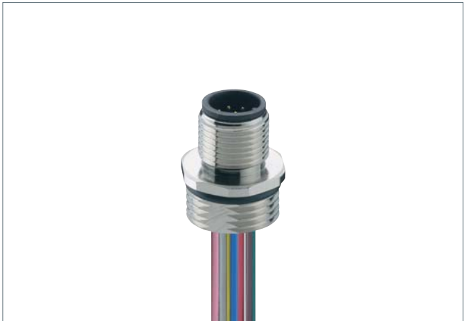
M12 panel mount connector, male, A-coded, IP67, for front mounting, thread M16, with stranded wires
