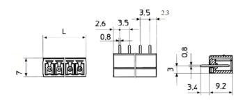
Closed headers Polarised mouldings Guided pin alignment
